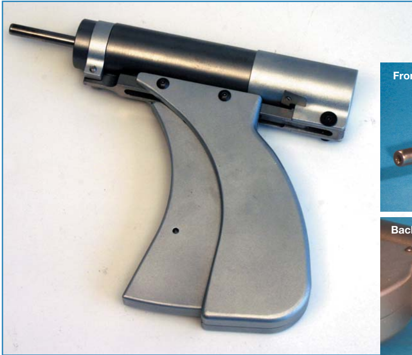
Fig. 1. Demonstration PowerCylinder™ set up with squeeze handles to mechanically drive internal pump. This unit has a ¼-in. ram rod and ⅜-in. bore; it can extend for 1¼ in.
